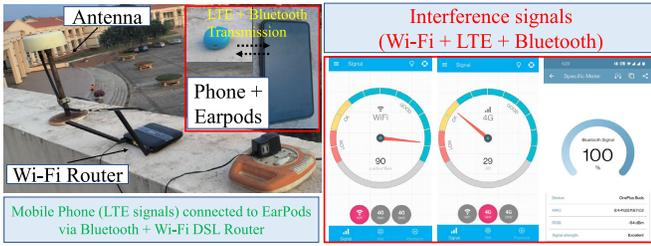
Fig. 4. Environment and instrumental setup of second test case: interference in urban canyon from Wi-Fi, LTE, and Bluetooth signals.
